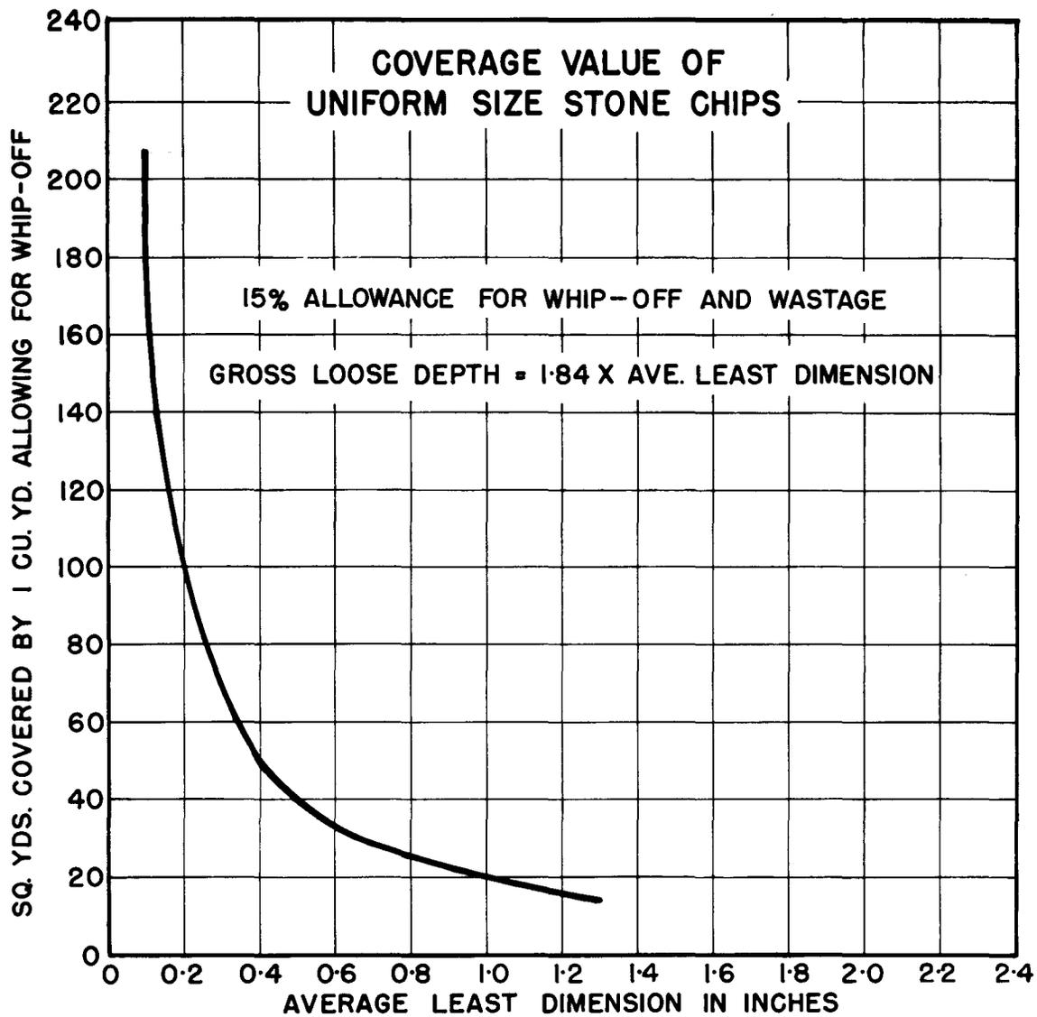
**FIG. 9 RELATIONSHIP BETWEEN AVERAGE LEAST DIMENSION AND COVERAGE VALUE WITH ALLOWANCE FOR WHIP-OFF AND WASTAGE.**
