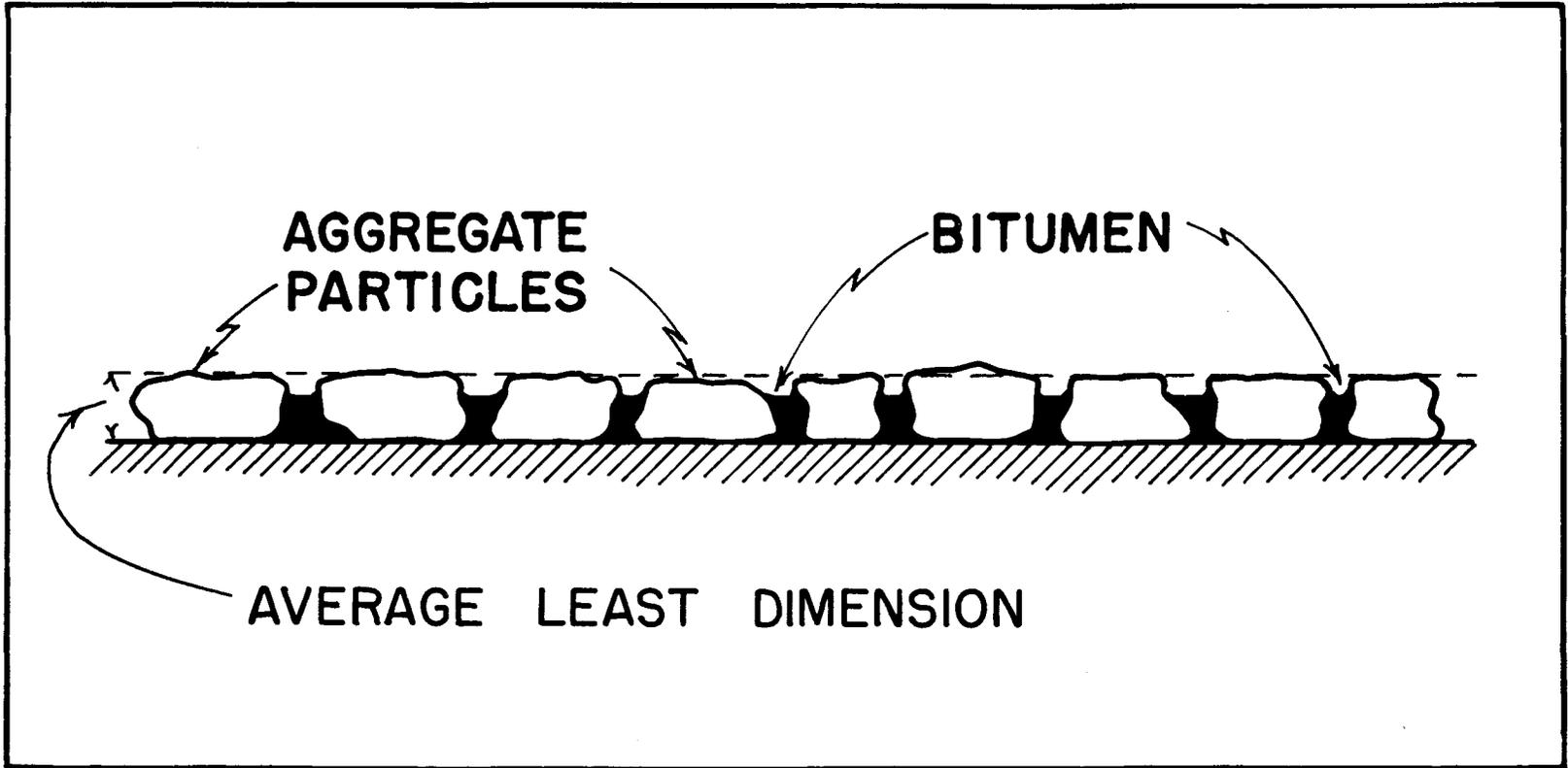
FIG. 7 PROPERLY CONSTRUCTED SURFACE TREATMENT OR SEAL COAT.
