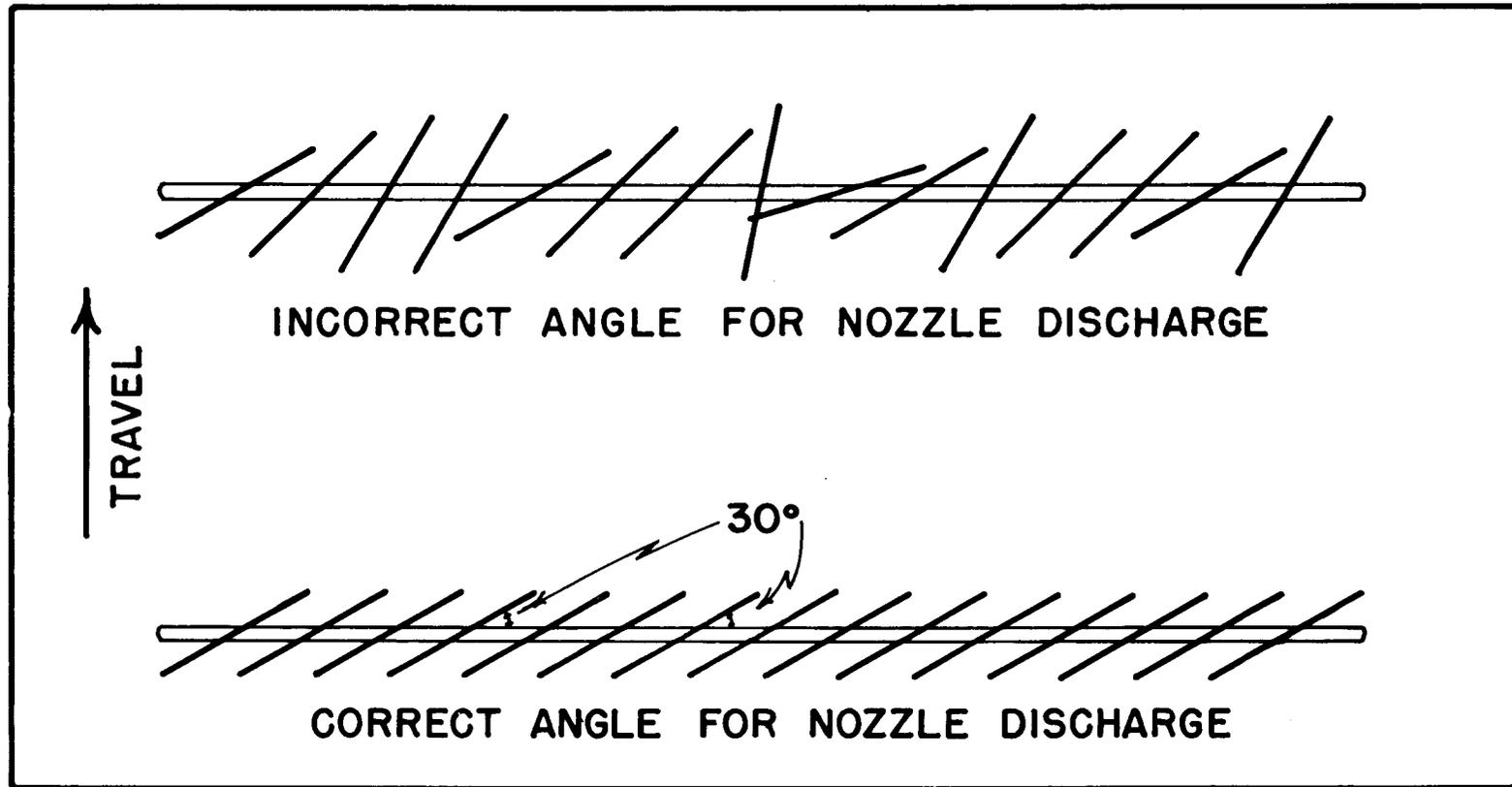
FIG. 1 INFLUENCE OF ANGLE FOR NOZZLE DISCHARGE.
