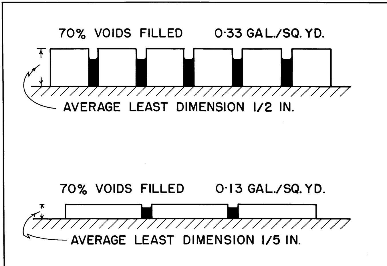
**FIG.12 COMPARING BITUMEN REQUIREMENTS FOR SEAL COATS MADE WITH 1/2 INCH COVER AGGREGATES OF DIFFERENT PARTICLE SHAPES — ONE CUBICAL, THE OTHER FLAT AND ELONGATED.**
