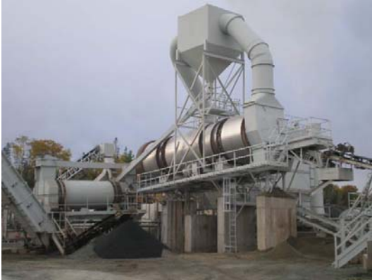
Pic 1: Dual drum counter flow plant: One drum to dry aggregate and one to mix. Equipped with baghouse.
